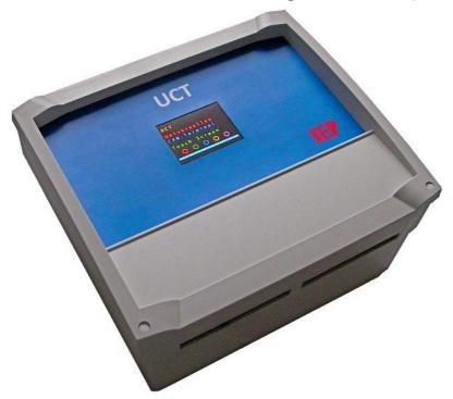
The **UCT** is a small controller for on-site mounting in low voltage equipment, e.g. for the control of heating and climate systems. For operating and visualisation, an OLED-display with a touch panel is integrated. With CAN as field bus, the UCT connects to a network and optionally controls additional I/O-modules.
