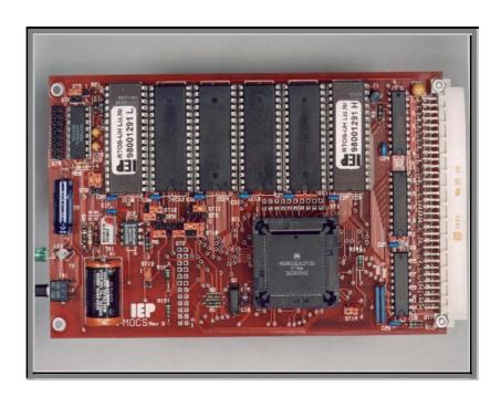
Based on the Motorola MC68332 microcontroller, the **MOCS** is a single board computer for the deployment stand-alone or as processor board in PBus systems.
