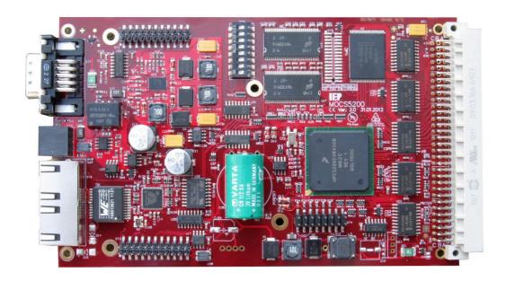
As a fast computing system, the **MOCS5200** is bound for demanding applications, requiring high computational power altogether with leading edge realtime reactivity. A 400 MHz PowerPC MPC5200 with integrated FPU, originally designed by the processor manufacturer for use in automotive multimedia systems, is the heart of the **MOCS5200** and delivers upto 700 MIPS.
