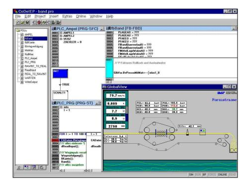
**CoDeSys** consists of two parts: a complete graphical PLC software development environment, runnable under Microsoft Windows opearating systems, and a PLC runtime kernel for the **RTOS-UH** realtime operating system. **RTOS-UH** guarantees for a stable and proven runtime environment for the **CoDeSys** kernel, featuring:
