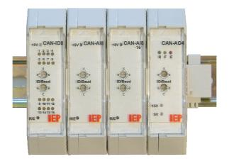
The CAN-xx modules are a line of durable and inexpensive I/O building groups for industrial control. A clear and sensible CAN communication structure simplifies their deployment. Optionally, the modules are available with CANopen® support.
